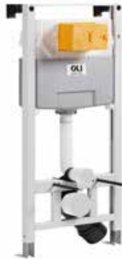
980cm Pre-wall, freestanding w.c frame including brackets and w.c bend with 3/6 litre dual flush plate front flush installation only.
