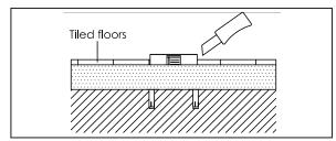
4.Pave the wood or gound tile and cut the exceeded part of the plastic box
