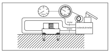
2.Make pressure test for the base union E190 by 10 hours in 10 bar to assure there is no any leakage befor the next step.
