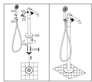
7.Take away the protective cover from the base union E190 and mount the poles E178 onto the base plate, locking with the nuts E192.Then slide down the cover E180 onto the floor.
