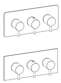
Concealed thermostatic shower valve three hole and two/three outlets
