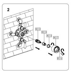
Check the 'o'rings for damage (ie. cuts or tears). Remove the 'o' rings before soaking the cartridge indescaling fluid. Soak the cartridge according to the instructions on the descaling fluid packaging. Rinseunder cold water before fitting (refer to the 'installing the thermostatic cartridge' section to install).
