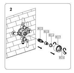
Check the 'o'rings for damage (ie. cuts or tears). Remove the 'o' rings before soaking the cartridge indescaling fluid. Soak the cartridge according to the instructions on the descaling fluid packaging. Rinseunder cold water before fitting (refer to the 'installing the thermostatic cartridge' section to install).
