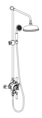
Grosvenor Exposed Thermostatic valve 2 outlets with Riser & Kit
