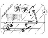
6.Adjust the top tube(2) Into a sultable height, lock the hand wheel until it is tight.
